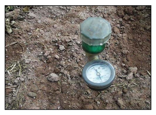
Tensiometers are effective tools to monitor soil moisture levels
