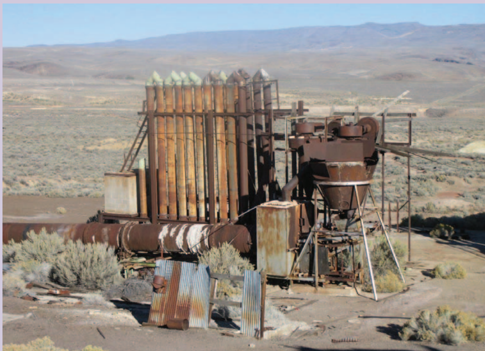
An old reduction furnace is one of the remnants of mercury mining near Eureka, Nev.
