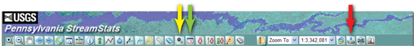
Figure 5–2. StreamStats toolbar. (Yellow arrow shows Basin delineation from a point , green arrow shows Obtain Basin Characteristics , red arrow shows Download option )
