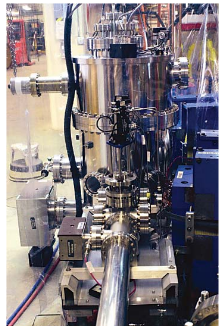
Jefferson Lab's free electron laser (FEL) - photo shows the vacuum container (silver cylinder) enclosing one of the mirrors at one end of the laser cavity.
