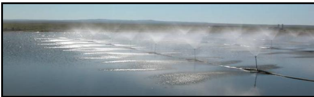
Figure 4: Sprays Used to Enhance Evaporation
