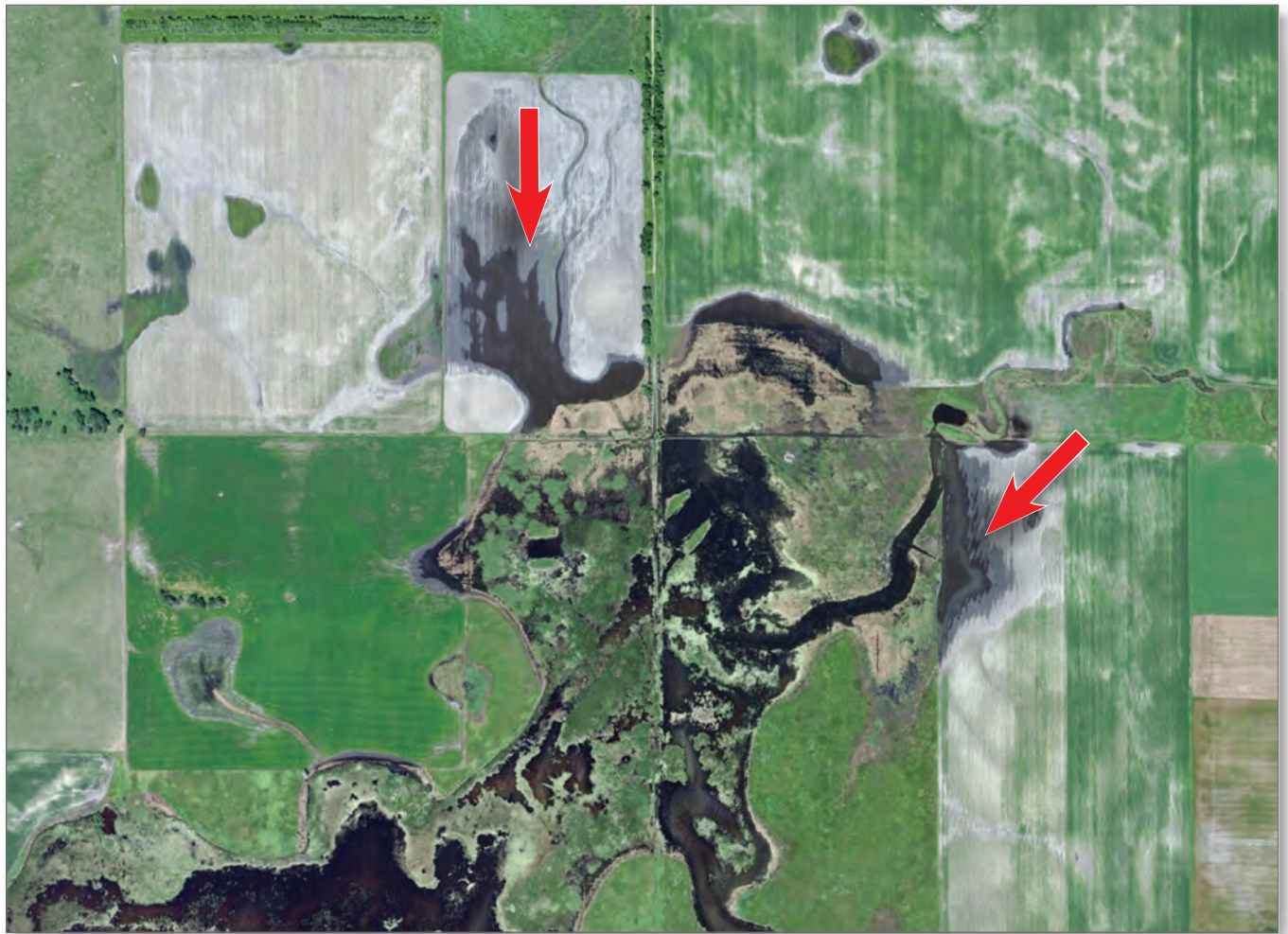
Figure 26. An example of wetland drainage into a larger wetland/water complex, Kingsbury County, SD, circa 2010. The red arrows show areas of former wetland that are being drained for agriculture. Dark gray and black tones are indications of wet soils as surface water is being removed. This type of drainage not only eliminates some wetland area but changes the hydrology of the wetland basin receiving the water being shunted off the landscape.
