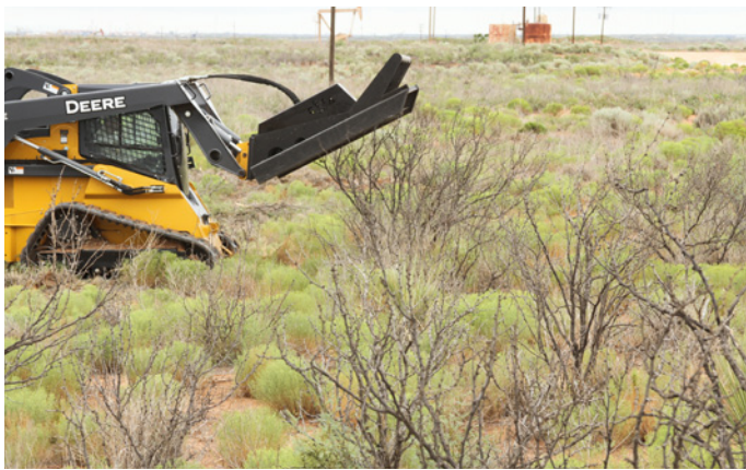
Two means of mechanically removing mesquite—mowing skeletons (above) and grubbing live plants. Grubbing can simultaneously kill mesquite and remove its vertical structure. Photo left: Randy Howard, BLM; photo right: Construction Equipment Guide.
