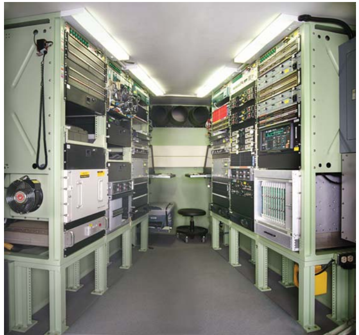
Above: The interior of the humvee shown at right containing the Marine Corps Joint Enhanced Core Communications System (JECCS) with Digital Tech Control (DTC) systems. JITC will conduct Joint Interoperability Certification tests of the JECCS with DTC systems during DICE '05.
