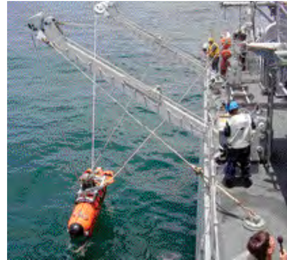
At sea aboard USS Champion (MCM 4) - Sailors aboard the mine countermeasures ship prepare to lower the AN/SLQ-48 "Mine Neutralization Vehicle" into the water. The remotely operated vehicle uses sonar and video cameras to find and identify underwater objects. If the operators find a mine, the vehicle can place small explosive charges near the mine to neutralize it. U.S. Navy photo by Lt. Marc Boyd.
