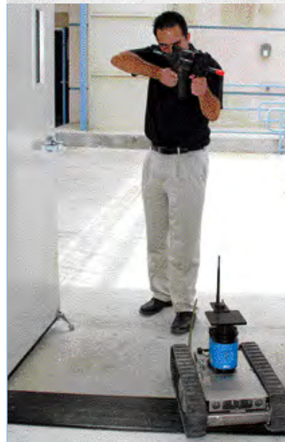
Top, controls engineer Brandon Sights follows the ARMS robot as it autonomously enters and maps a building. In the photo below, the ARMS prototype, based on iRobot's PackBot, automatically assumes a defensive screening maneuver between Sights and the perceived threat.
