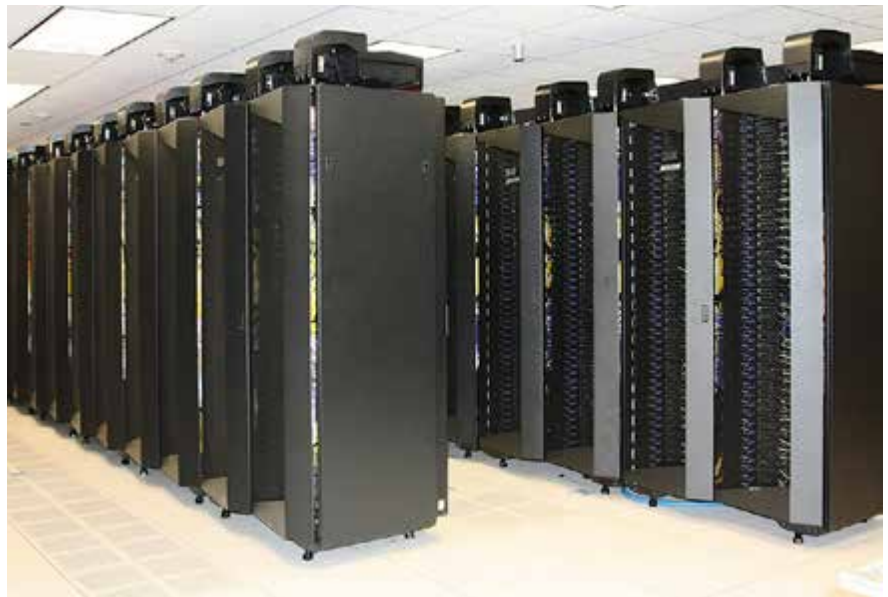
The Navy DoD Supercomputing Resource Center (DSRC) is home to three IBM iDataPlex supercomputers with a total theoretical peak performance exceeding 954 teraflops (trillion calculations per second). This world class scientific computing environment provides the capability for DoD scientists and engineers to accelerate delivery of new technologies and for the Naval Meteorology and Oceanography Command to deliver oceanographic products that support the safety, speed and operational effectiveness of the fleet. Photo courtesy of Navy DSRC by Lynn Yott.
