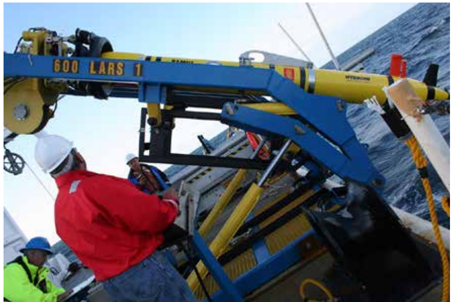
NORTH SEA (Sept. 17, 2010) Naval Oceanographic Office surveyors John Suslavage and David Small prepare to launch autonomous underwater vehicle, REMUS 600 aboard the Military Sealift Command oceanographic survey ship USNS Henson (T-AGS 63). They are in search of the remains of John Paul Jones' Revolutionary War ship Bonhomme Richard, which was lost off the coast of England in 1779 after a decisive battle with HMS Serapis. Jones won the battle and seized HMS Serapis as Bonhomme Richard was heavily damaged and sank 36 hours later. U.S. Navy photo by Rebecca Burke.
