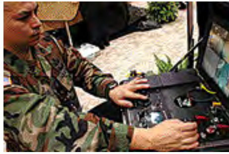
U.S. Army Staff Sgt. Santiago Tordillos operates the armed robotic system, SWORDS, by remote control with two joy sticks on a control panel, tracking where it’s going on a small screen. U.S. Army photo by Sgt. Lorie Jewell.
