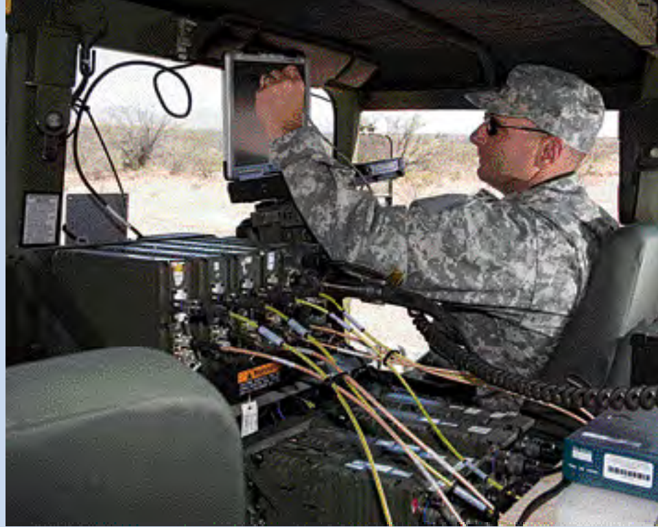
The Joint Interoperability Test Command (JITC) testing of the Ground Mobile Radio (GMR) at Fort Huachuca. The GMR is designed for vehicles and is an integral part of the Army Future Combat System for networking. All JTRS-approved radios must be JITC-tested for interoperability with legacy radios, as well as new wave forms. They must also meet National Security Agency security standards. Photo courtesy of Boeing Corp.
