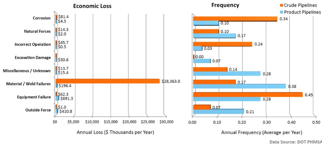
› The leading event type affecting **crude oil pipeline and petroleum product pipelines** in Michigan during 1986 to 2014 was **Equipment Failure** for crude oil pipelines and **Material/Weld Failures** for product pipelines, with an average **0.45 and 0.38 incidents** per year (or one incident every 2.2 and 2.6 years), respectively.
