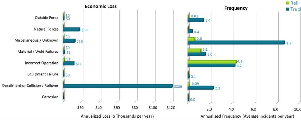
› The leading event type affecting the **transport of petroleum product by rail and truck** in Michigan during 1986 to 2014 was **Incorrect Operation** for rail transport and **Miscellaneous/Unknown** for truck transport, with an average **4.3 and 8.7 incidents** per year, respectively.
