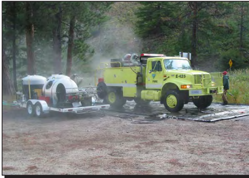
Plate 2.15: The MDTC portable vehicle washer being used in the field.
