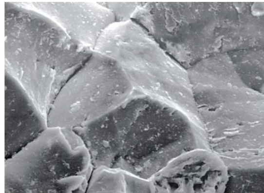
Fig. 4 — Intergranular fracture due to hydrogen embrittlement (photo courtesy of Aston Metallurgical Services Co., Inc.).
