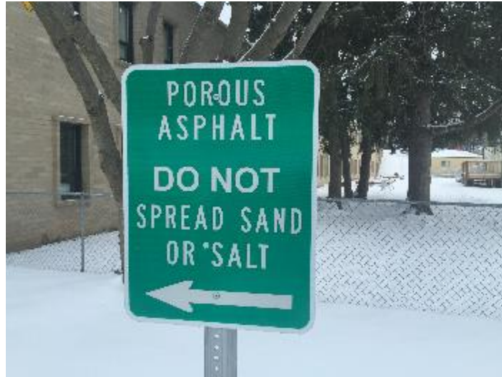
Exhibit 14-9. Porous Asphalt Signage (Credit: Tetra Tech)
