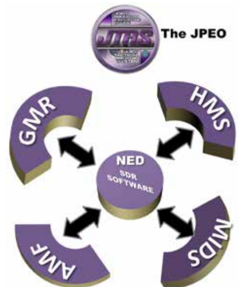
FIGURE 2. STRUCTURE OF THE JTRS PROGRAM GMR: GROUND MOBILE RADIO (NOW MID-TIER NETWORKING VEHICULAR RADIO (MNVR)); HMS: HANDHELD, MAN-PACK & SMALL FORM FIT; MIDS: MULTIFUNCTIONAL INFORMATION DISTRIBUTION SYSTEM RADIO;AMF: AIRBORNE/MARITIME FIXED RADIO.
