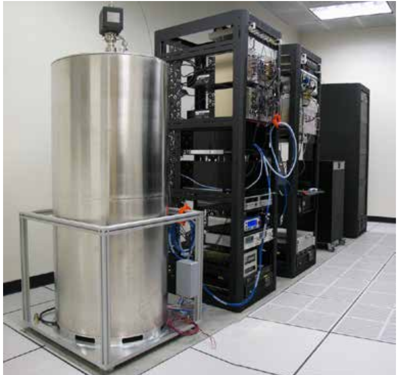
The Navy Rubidium Fountain Clock No. 3, one of four such devices that are now part of the Master Clock system. This device and its companions are the most precise clocks currently operating in the world. All USNO photos by Geoff Chester/USNO public affairs officer.
