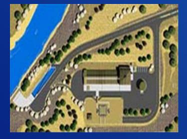
Water from Animas River pumped into Lake Nighthorse through the Ridges Basin Inlet Conduit – 72-inches diameter & 2.1 miles long buried pipeline.
