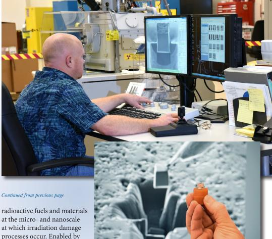
radioactive fuels and materials at the micro- and nanoscale at which irradiation damage processes occur. Enabled by its modular design, IMCL will continue to evolve and improve capability to meet the national and international user demand for high-end characterization instruments for the study on nuclear fuel and materials.
