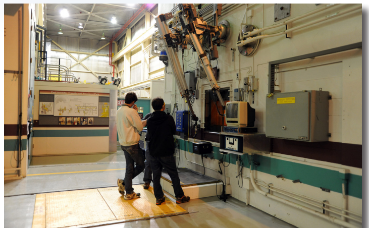
FCF is equipped with heavily shielded hot cells and remotely operated manipulators, which enable researchers to safely handle irradiated fuels and materials.
