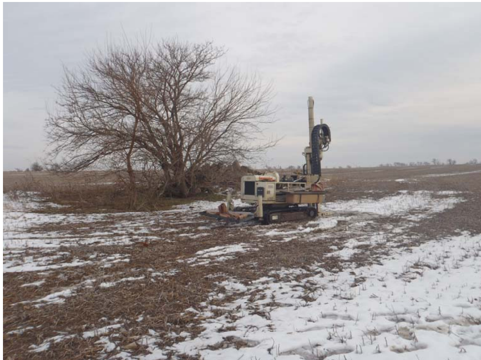
Site: York Township Dump Site Photograph No.: 2 Direction: Southeast Subject: View of Geoprobe drilling operations at soil boring location YD-B01
