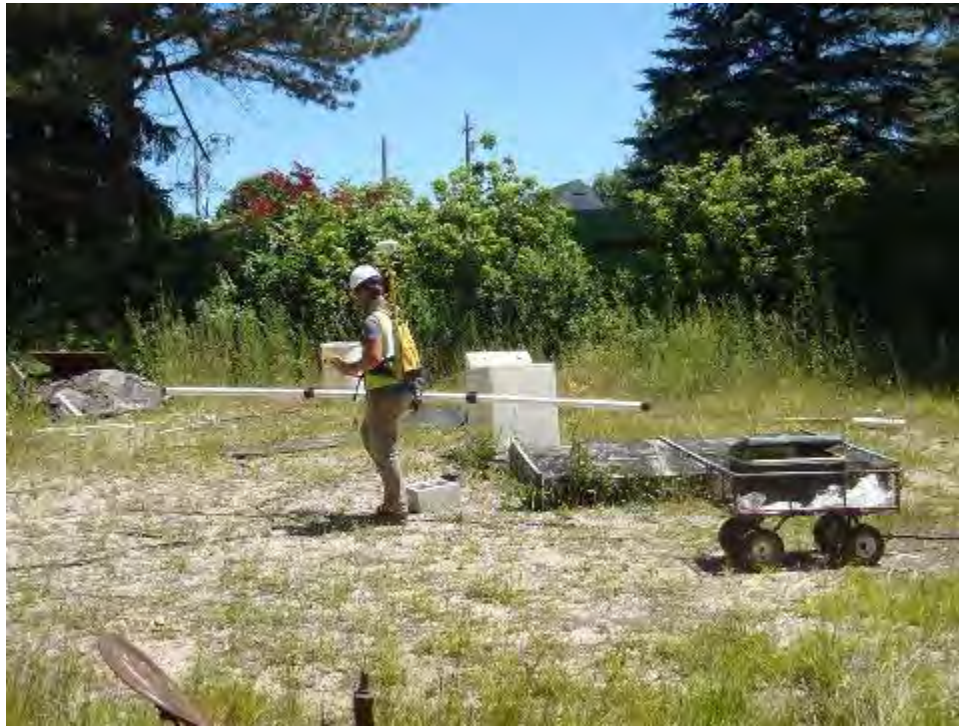
Site: Clyde Paint and Supply Company Site Photograph No.: 9 Direction: South Subject: EM survey in fenced southern portion of Site
