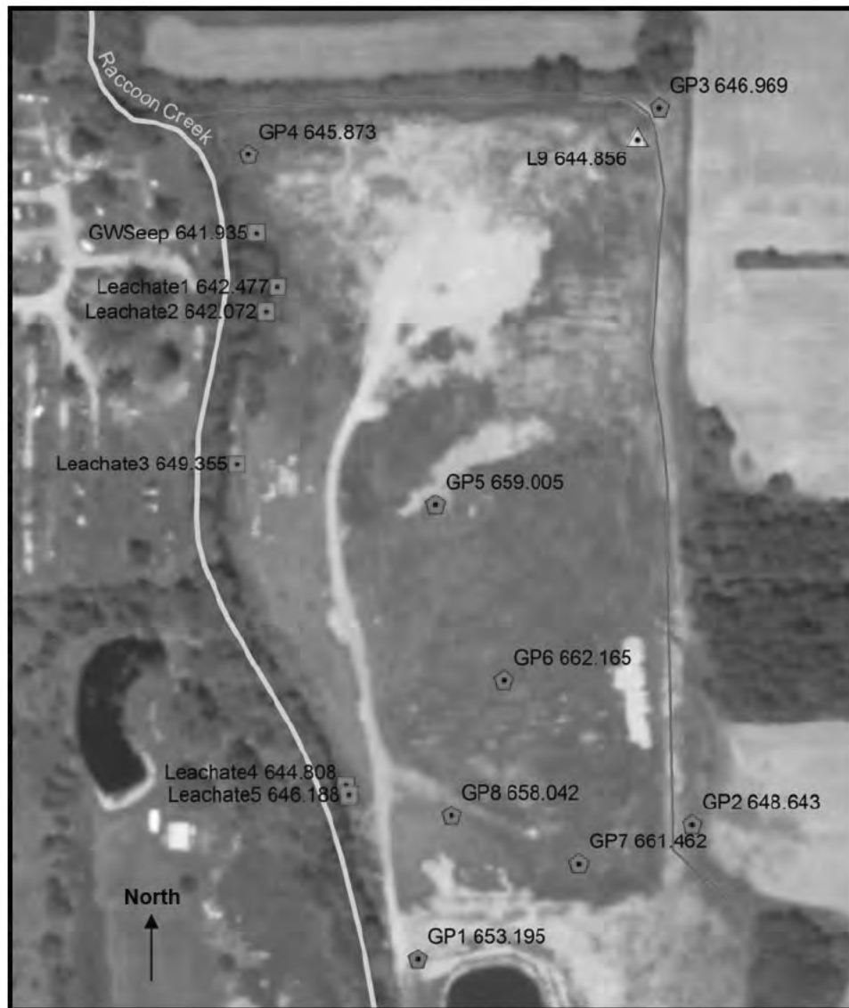
Figure 3: Site map showing the surface elevations of the boring locations (GP) and leachate/ground water seeps. Raccoon Creek ranges in elevation from 641.5 in the southern upstream portion to 638.1 in the northern downstream portion onsite. Elevations are in feet above mean sea level (ft AMSL).
