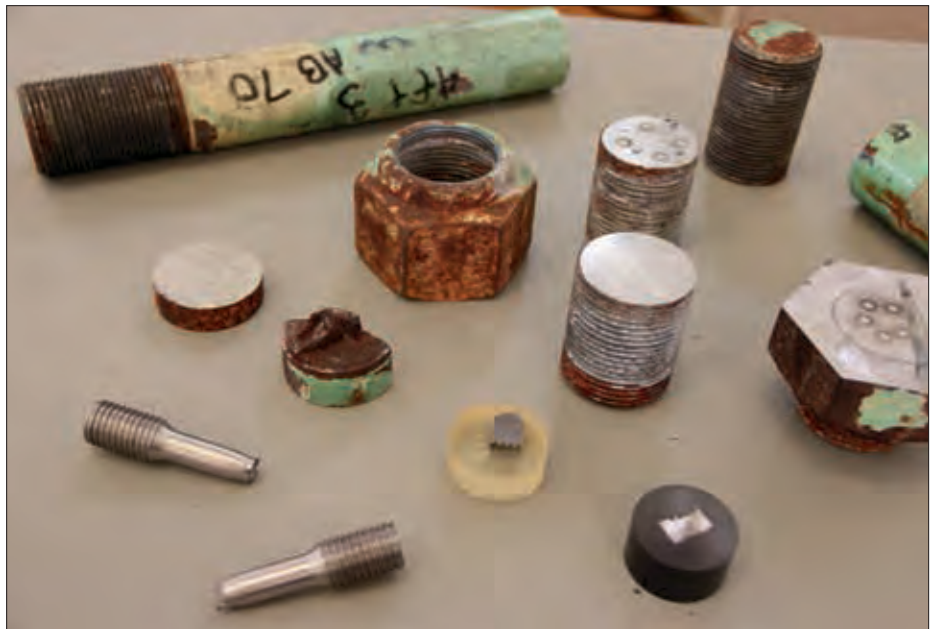
BSEE’s Interagency Bolt Action team is examining the issue of offshore subsea bolt failures. The team has representatives from a dozen federal agencies and research labs whose areas of expertise involve subjects such as metallurgy. BSEE’s goal is to determine why bolts are failing in ways that are not expected. BSEE’s goals are to determine what is going wrong and how to fix it before a catastrophic event occurs.
