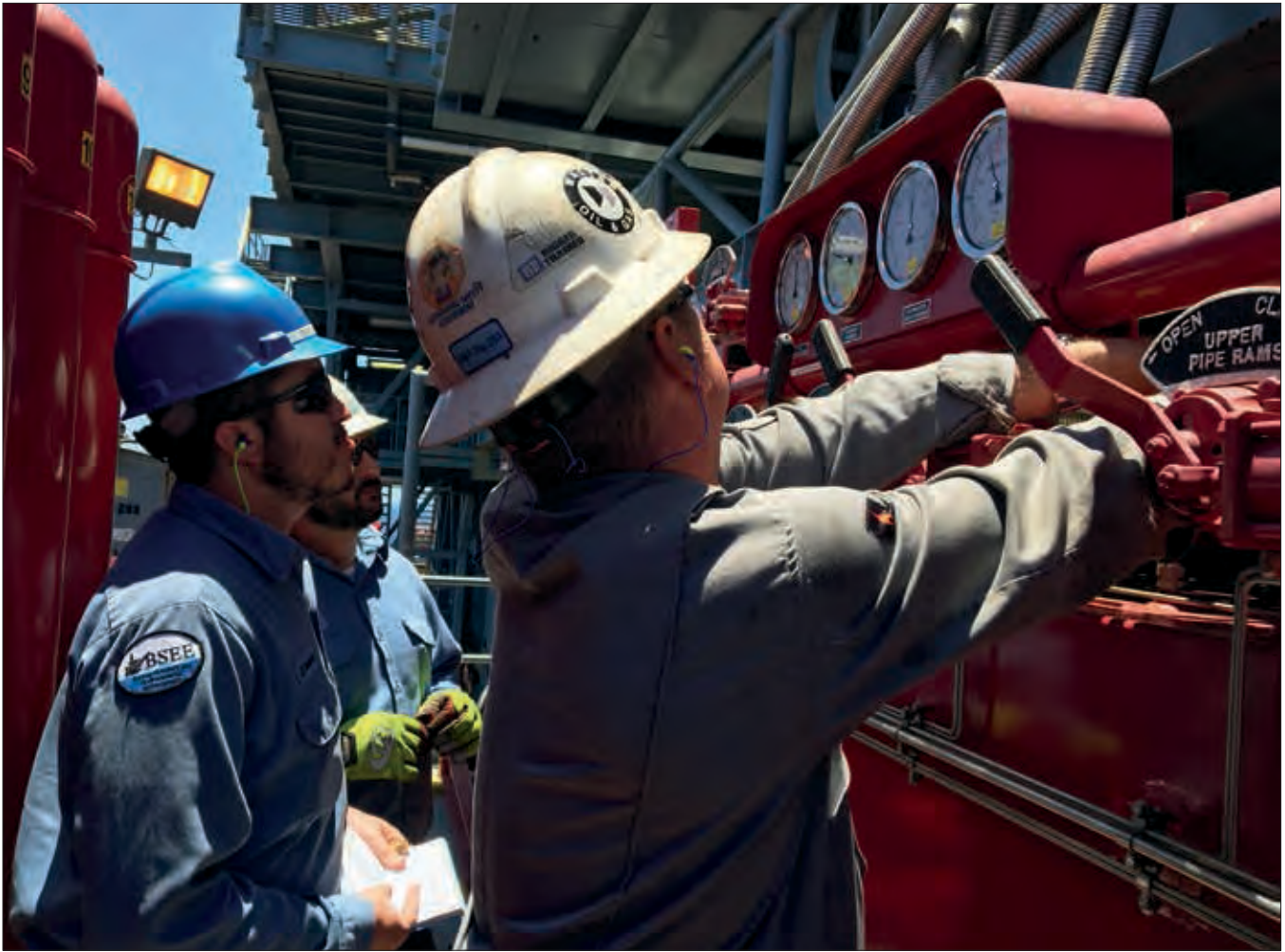
Inspectors from BSEE's New Orleans District Well Operations Unit observe the company's tool pusher as he conducts a successful test of the facility's accumulator.
