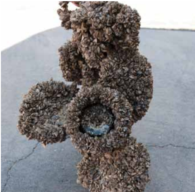
The colonization of quagga mussels can be seen on this boat propeller recovered from Lake Mead.
