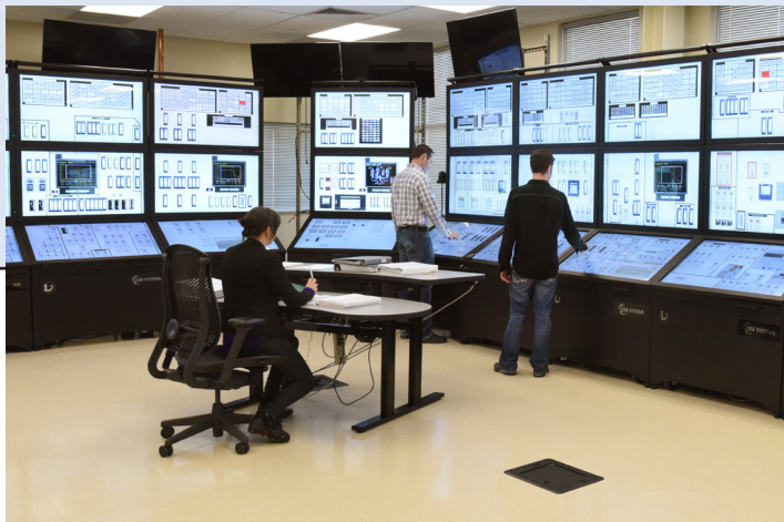
The HSSL facility enables INL scientists to safely and cost-effectively develop and evaluate new control room technologies with actual operators in a representative setting.
