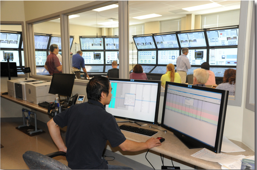
HSSL training evaluators and human factors researchers can observe, record and study operator performance and introduce changing scenarios in real time.
