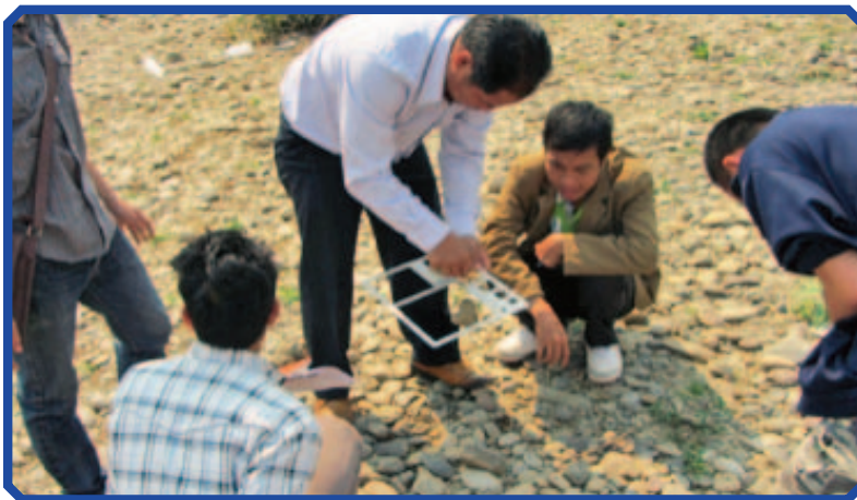
Laos trainees taking pebble count measurement to assess sediment grain size distribution.
