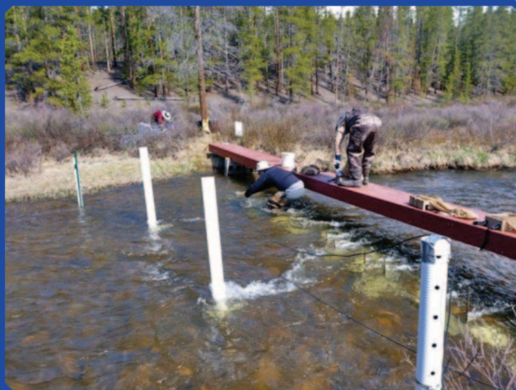
Installing Bunte bed load traps immediately downstream of two hydrophones on Halfmoon Creek, Colorado. The hydrophones are installed near the bed using posts and hydrodynamic fairings.
