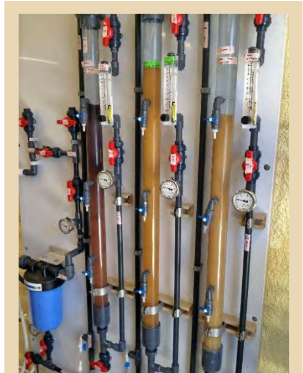
Top: Pilot-scale ion exchange columns. Bottom: Regeneration brine.
