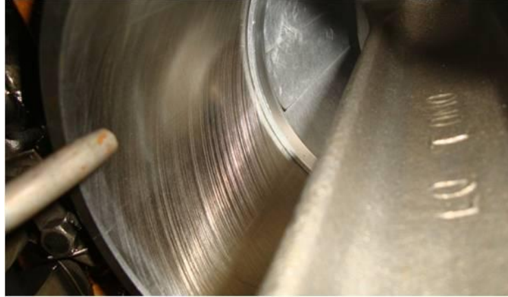
Figure 29. Cylinder Number 6 -Lower End Hone Marks
