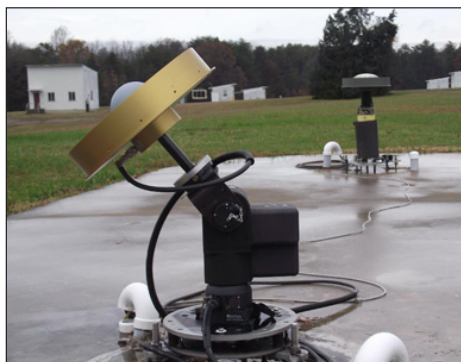
Absolute antenna calibration at NGS' Corbin, Virginia, facility. A robot, foreground, rotates the tested antenna through multiple orientations to measure phase delays.
