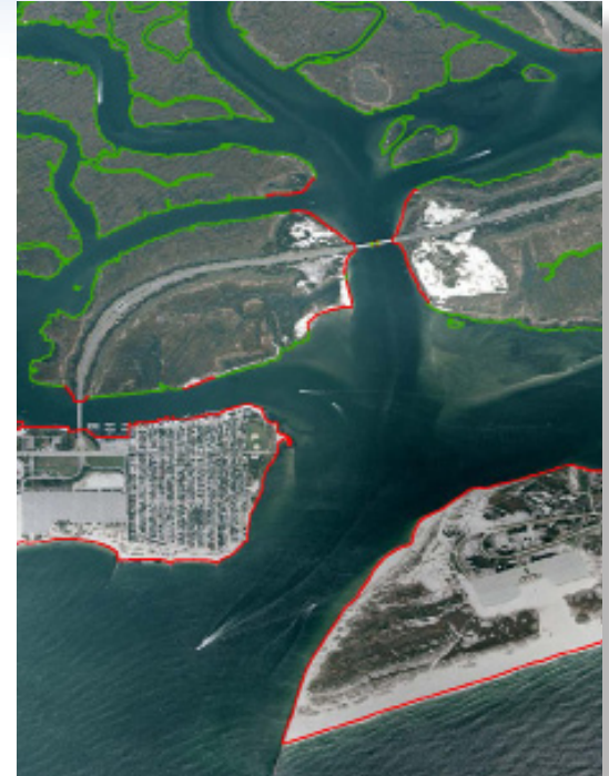
Image of Jones Inlet, Long Island, NY using Applanix Digital Sensor System. The green line represents marsh (apparent) shoreline, and red line represents mean-high water shoreline.
