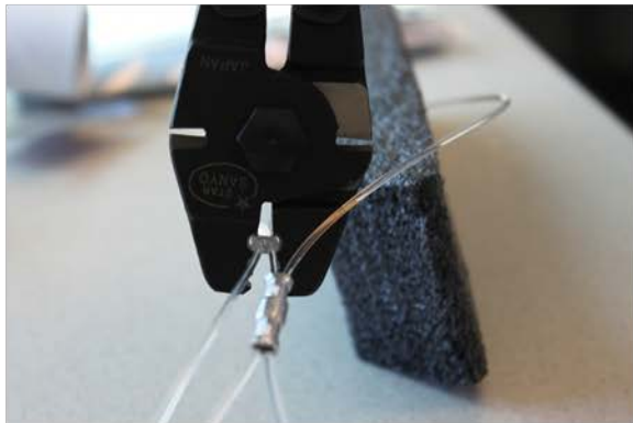
Figure 4. Bring both ends of the monofilament through the crimp sleeve in opposite directions and crimp on both ends.
