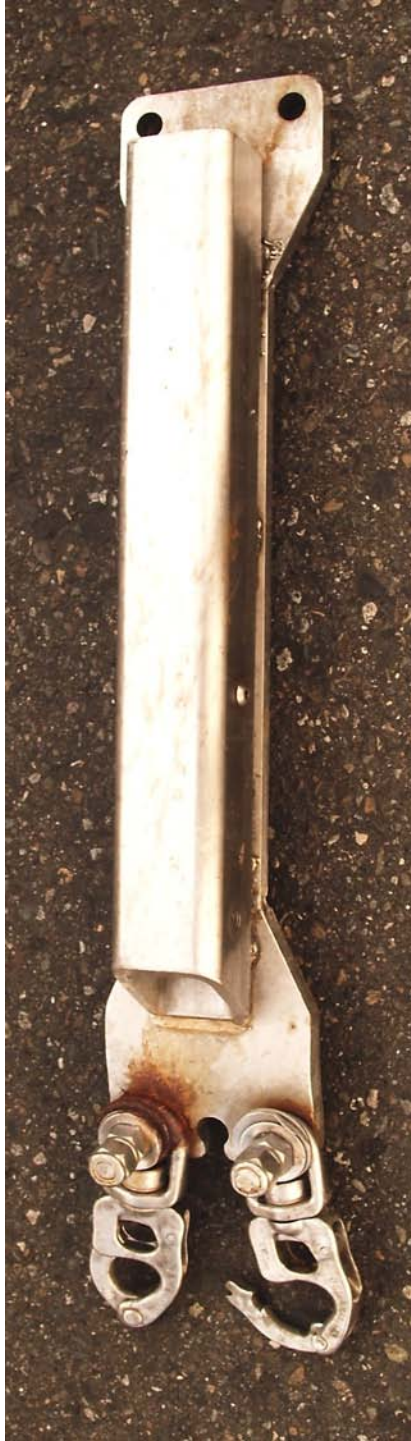
Figure 2f. - - Photo of the bottom contact sensor and its footrope attachment configuration to the ground gear used during the 2010 EBSS survey.
