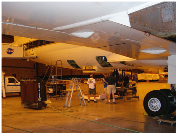
Figure 46: University of Kansas MCoRDS antenna system is integrated to the DC-8 in preparation for Antarctic Operation ICE Bridge mission.
