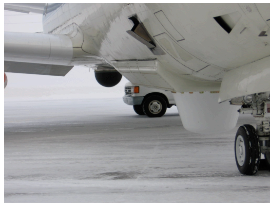
Figure 15: P-3 belly, PALS installed in the forward white radome, PolSCAT in the aft black radome.
