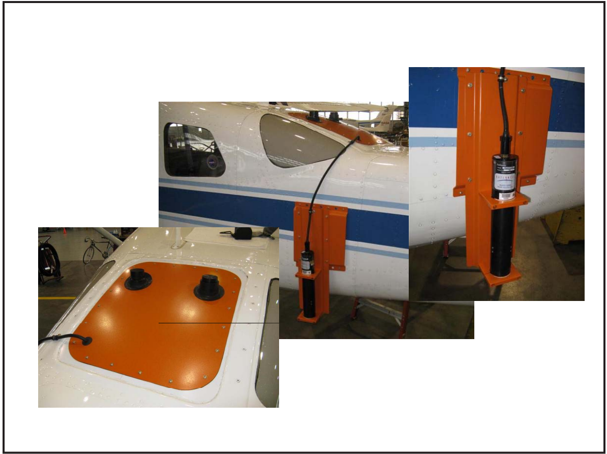
Figure 13: Installation of the three EPA hyperspectral ocean color radiometers on the NASA Cessna 206H aircraft.
