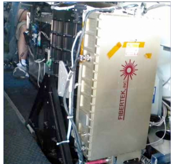
Figure 32: A High Spectral Resolution Lidar and Research Scanning Polarimeter are located within the King Air.
