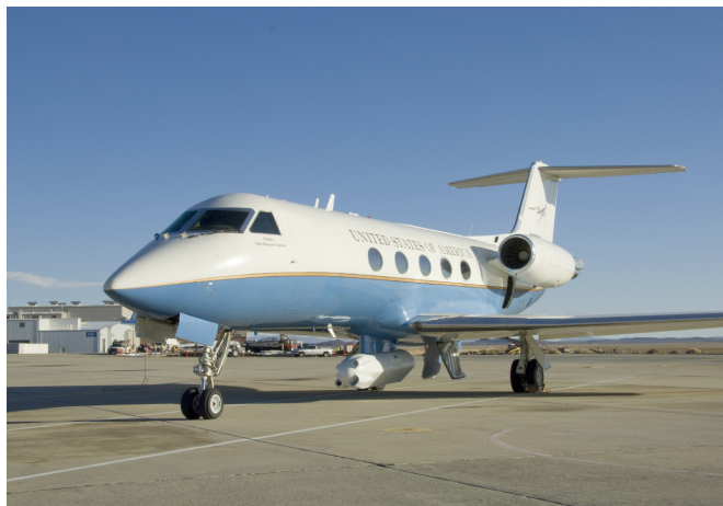
Figure 8: UAVSAR mounted under the G-III at Dryden Flight Research Center.
