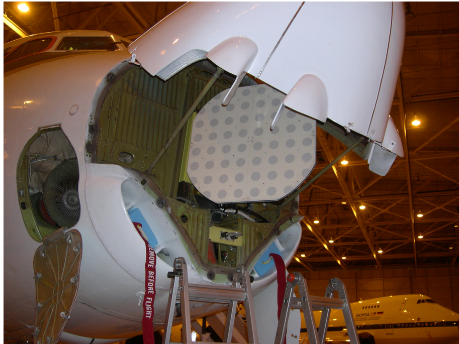
Figure 44: Ktech TM data receiving antenna mounted in nose of DC-8 supporting NASA/USAF Vandenberg, CA rocket launch TM Relay Mission. The SOFLA aircraft is in the background.
