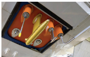
Inlets on the belly of the NASA B-200 collect samples of carbon and methane during flight.
