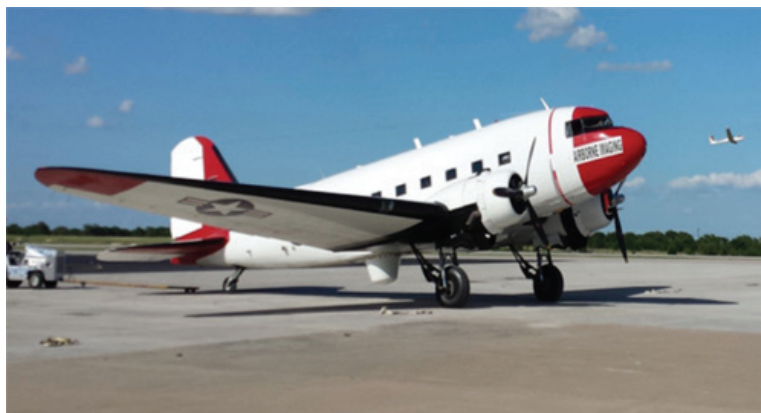
Airborne Imaging Inc., N737H DC-3 with the PALS radome underneath the aircraft
