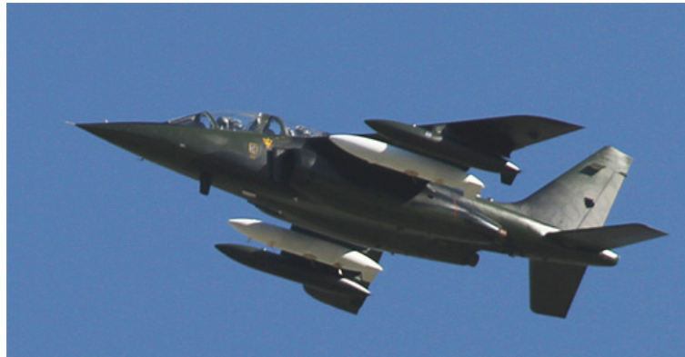
The Alpha Jet, based at Moffett Field, carries the AJAX payload in two unpresurized wing-mounted sensor pods. The trace-gas payload measures ozone, formaldehyde, carbon dioxide, methane, water vapor, and three-dimensional winds. Available window ports can be seen on the underside of each white sensor pod.
