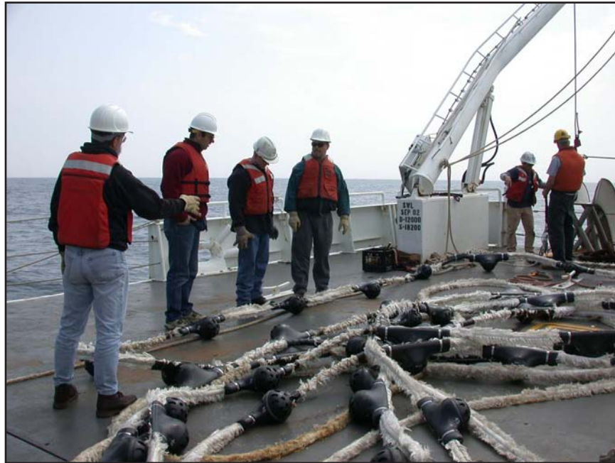
Preparing 64-element source/receive array for deployment
