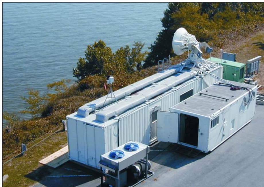
Shelters housing the high-power 94 GHz radar
