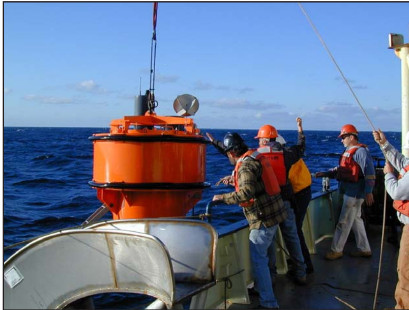
Surface telemetry buoy connected to a 64-element acoustic receiver
