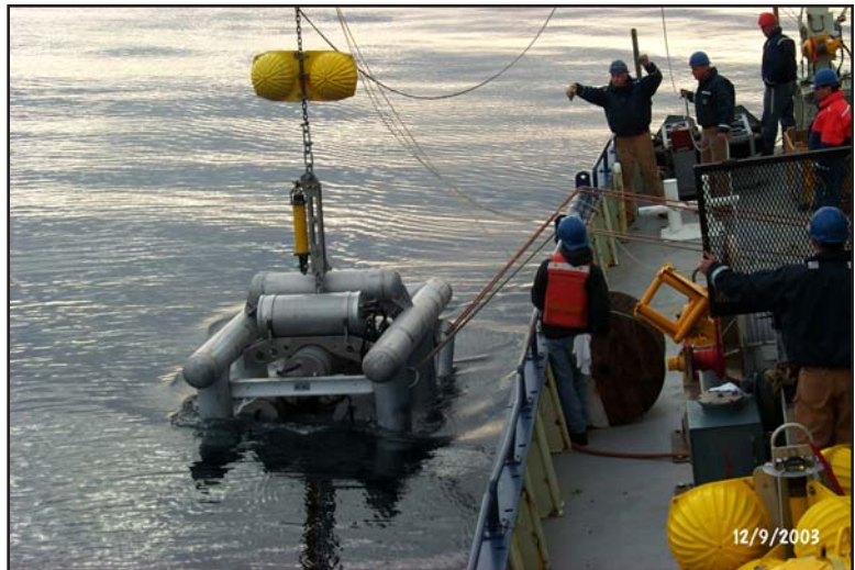
Deployment of instrumentation sled for 96-element acoustic horizontal line array receiver system
