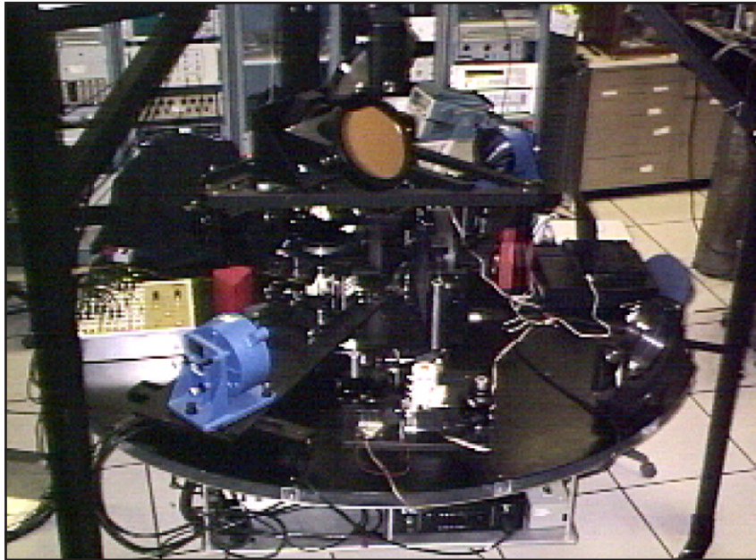
Open-loop rate table for hardware IRCM testing
