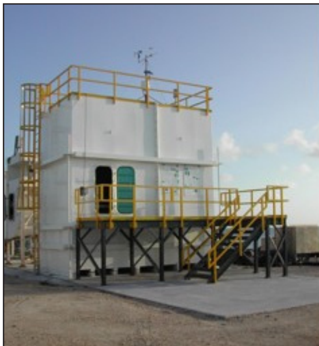
Ship ballast tank mock-up at the Ballast Water Treatment Test Facility
