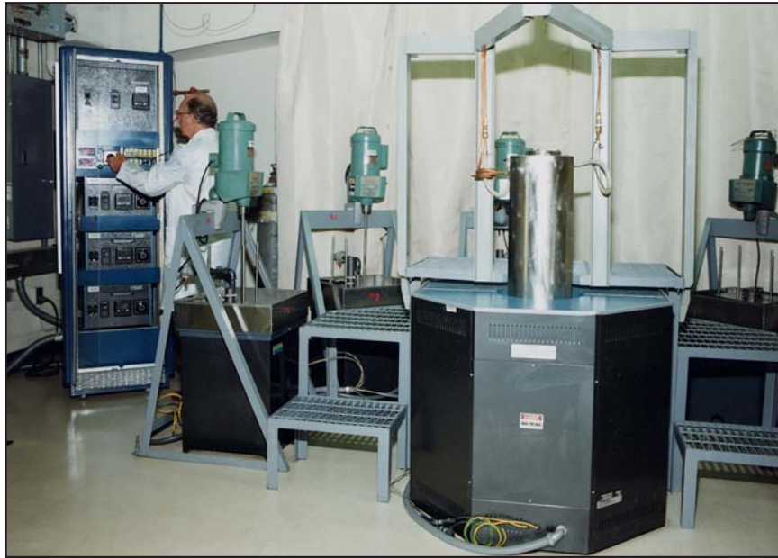
Isothermal heat treatment facility
