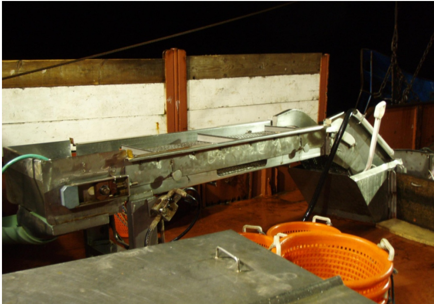
Figure 71. Conveyor belt with checker pen (on right) and discard chute (on left).
