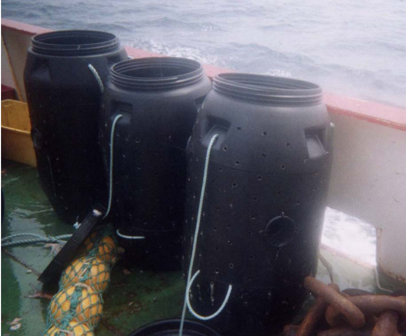
Figure 13. Hagfish pots showing escape vents.
