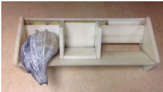
Figure 87. An example of how to obtain width measurements using the Whelk Sampling board.
