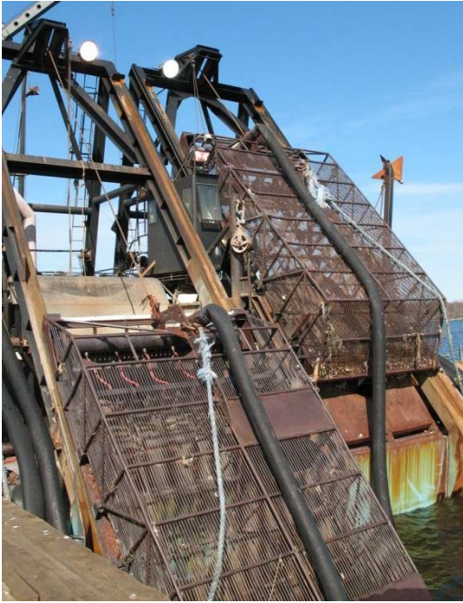
Figure 45. Example of a tow line attached to a dredge.
