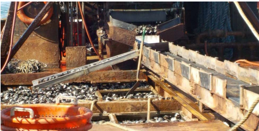
Figure 49. An example of a conveyor system set up to fill a specific section of cages on deck.
