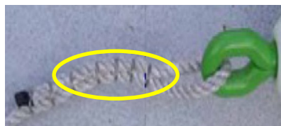
Hog Rings: metal crimps that connect the line and part under a load
