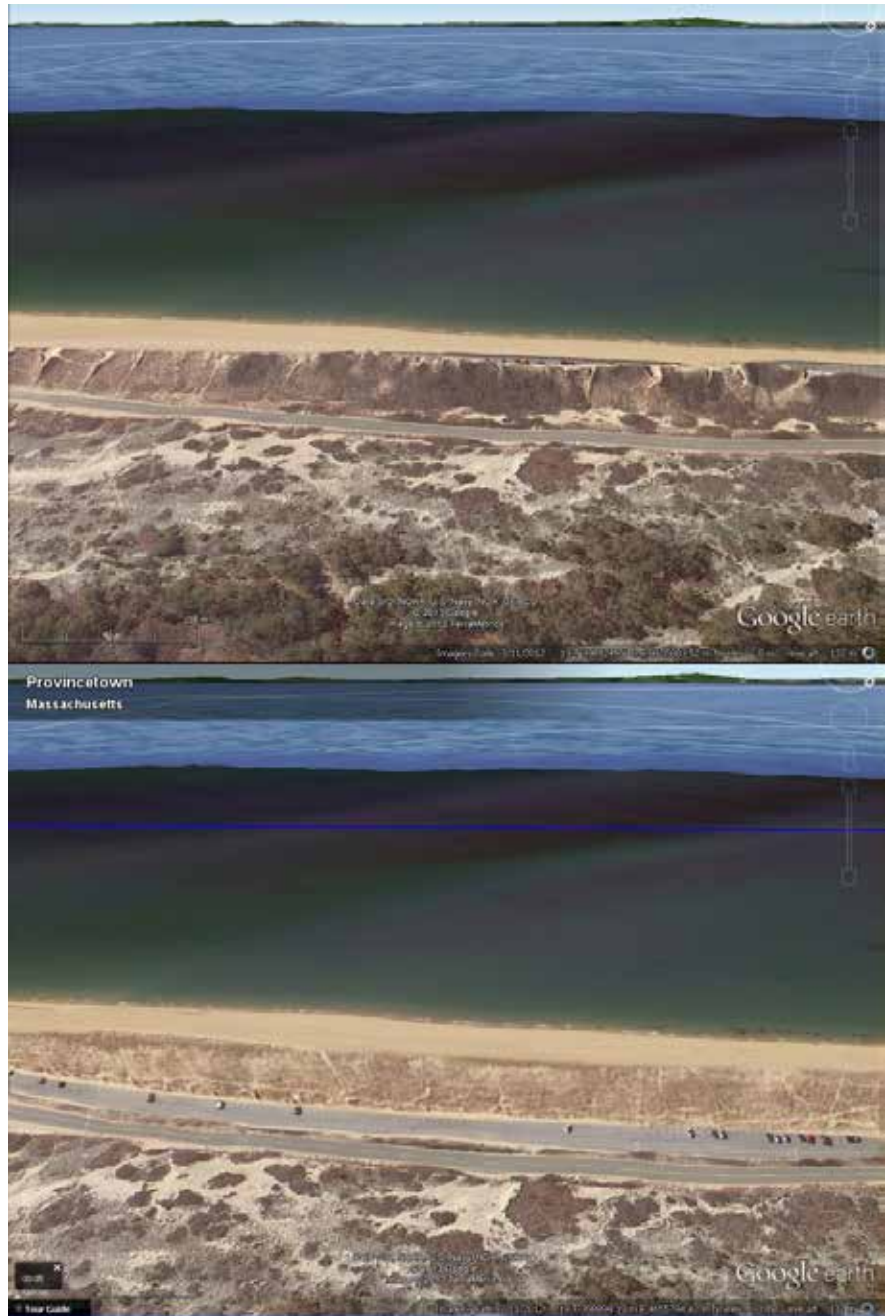
Top: Before the Herring Cove redesign, visitors parked between the beach and an artificial dune. Image credit: Google Earth. Bottom: Following the redesign, the parking lot will be adjacent to the road, and the artificial dune will be reshaped to mimic adjacent natural topography. Image credit: Mark Adams (NPS) conceptual visualization using photographs from Google Earth.
