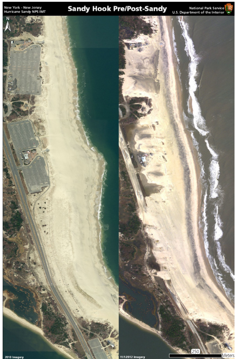
Figure 6.1. Built facilities, also known as assets, including roads, parking lots, and buildings, such as these pictured before and after Hurricane Sandy at Sandy Hook unit of Gateway National Recreation Area in New Jersey, are vulnerable to rising water level. In the post Sandy image, sand covered the parking lots.
