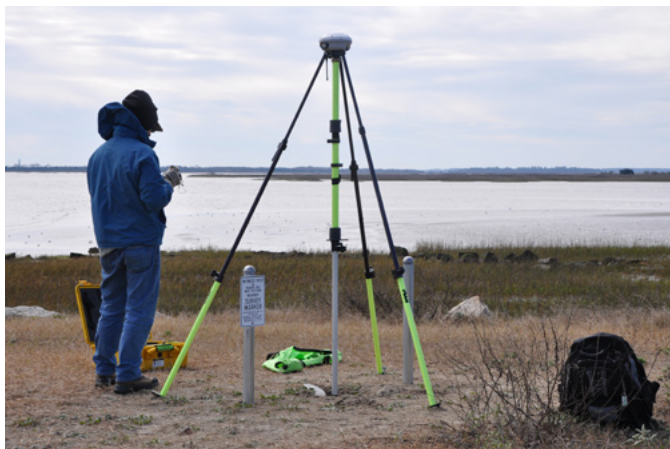
Figure 6.4. Image of base station set up for RTK-GPS elevation data collection at Fort Sumter National Monument as part of the vulnerable asset elevation project in 2015.
