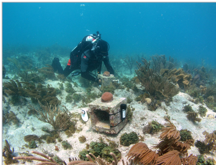
USGS diver working on the calcification blocks at Biscayne NP. A temperature logger is seen on the block in the foreground. Photo Credit: Ilsa Kuffner, USGS
