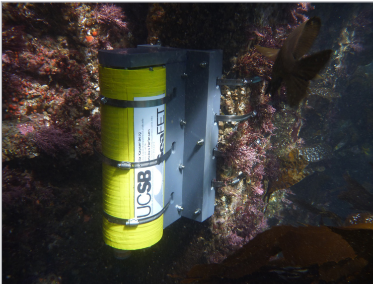
SeaFET ocean pH sensor deployed on the pier at Anacapa Island. NPS photo by David Kushner
