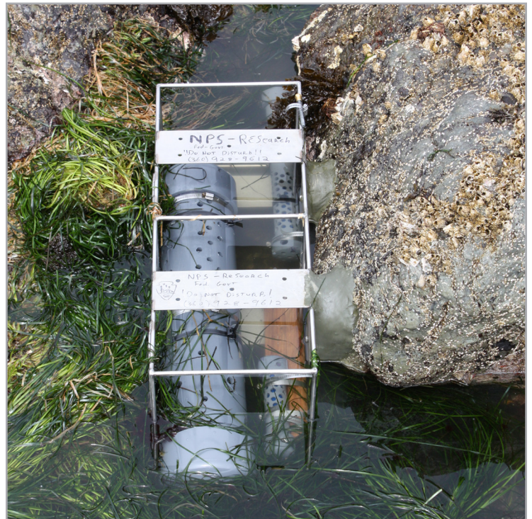
The OA monitoring instrument package installed in a tidepool in the American Camp unit of SAJH. NPS Photo
