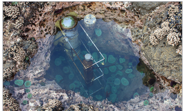
The OA monitoring instrument package installed in a tidepool at Sokol Point, OLYM. This package includes newer SeaFET™ instrumentation (inside cage), and the Collocated older multiprobe datasonde that will be phased out in 2017. NPS Photo
