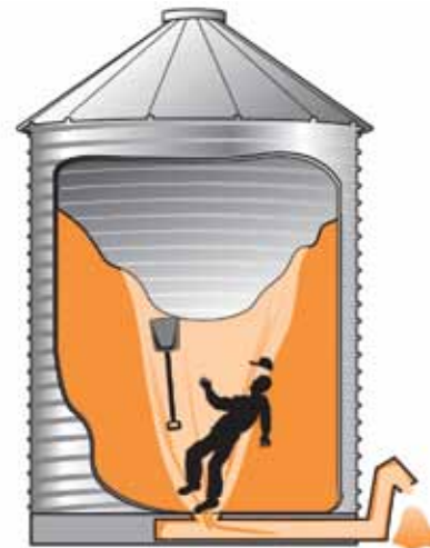
A center grain unloading auger draws grain from the top center and the grain forms a cone as the bin is emptied.
