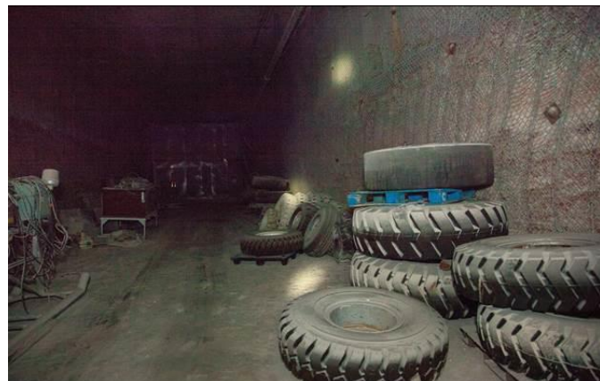
Figure 17: Combustible Loading in the Mine
