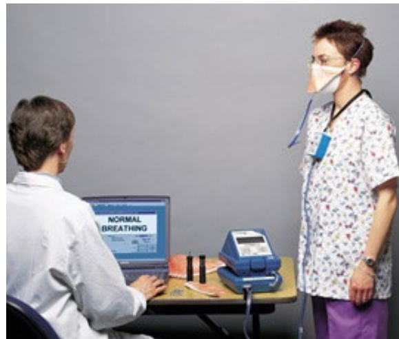
Worker receiving quantitative fit testing.
