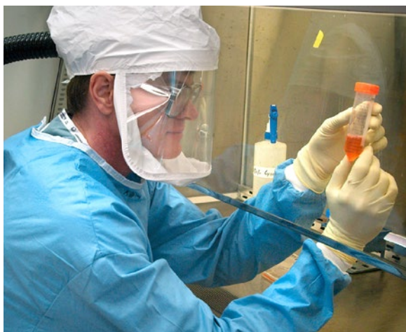
Laboratory worker wearing powered air-purifying respirator.
