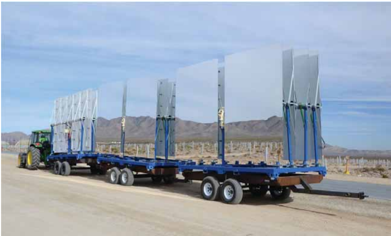
Power tower heliostats on trailer enroute to installation. Heliostat backs are visible on reversed heliostats at front of trailer. Heliostat supports are visible in heliostat reflections and to the right of the trailer. (Credit: Robert Sullivan, Argonne National Laboratory.)
