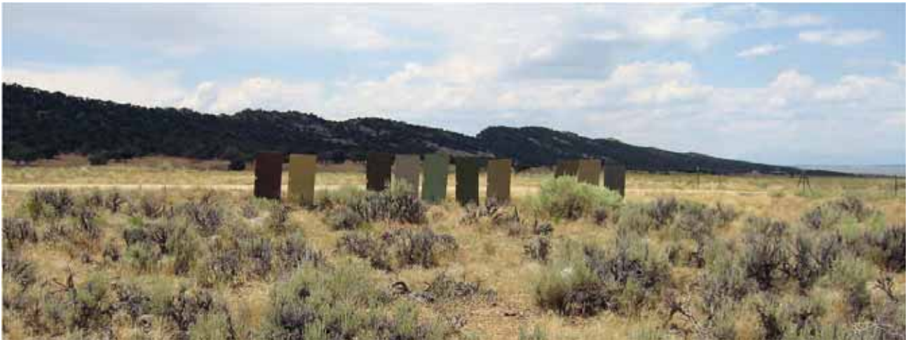
BLM standard environmental color panels are used to identify the best match between facility colors and the surrounding landscape. (Credit: BLM.)
