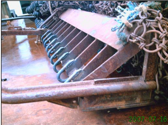
Figure 3. Side view of shoe used; the shoe was \frac{1}{2} " x 3" spring steel cut 17 \frac{1}{2} " long and attached to 1 \frac{1}{2} " x 3 \frac{1}{2} " x 15" long bar stock
