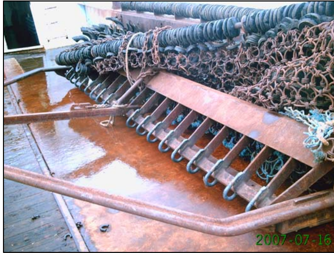
Figure 1. Experimental dredge design 3 with turtle guards on the cutting bar and a doubled outer bale.
