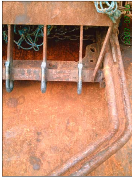
Figure 5. The bale extended forward 9 inches (interior measurement) before tapering to the tow point.
