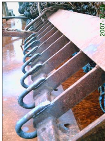
Figure 4. Space between struts measured 8 \frac{1}{2} "; the spacing between the 8" depressor plate and cutting bar measure 10". The turtle guards were made of 1" hardened steel round stock and placed every 9" along struts
