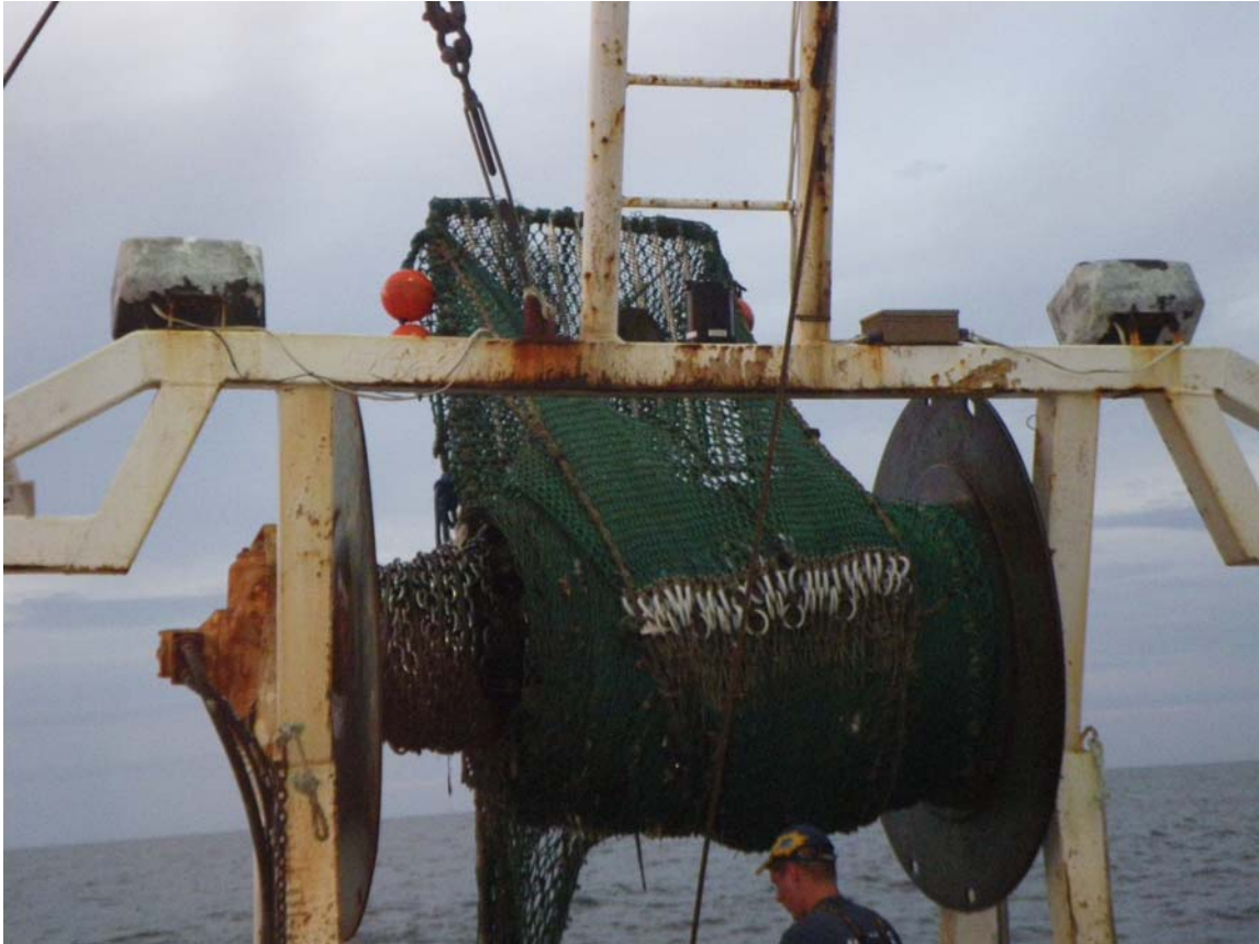
Figure 18. Typical LF-TED position on net drum during haul-back.
