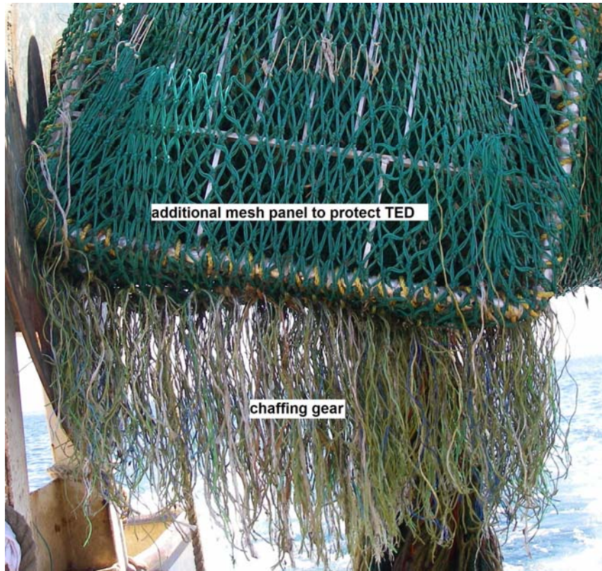
Figure 17. Chaffing gear added to protect wearing of the extension meshes.
