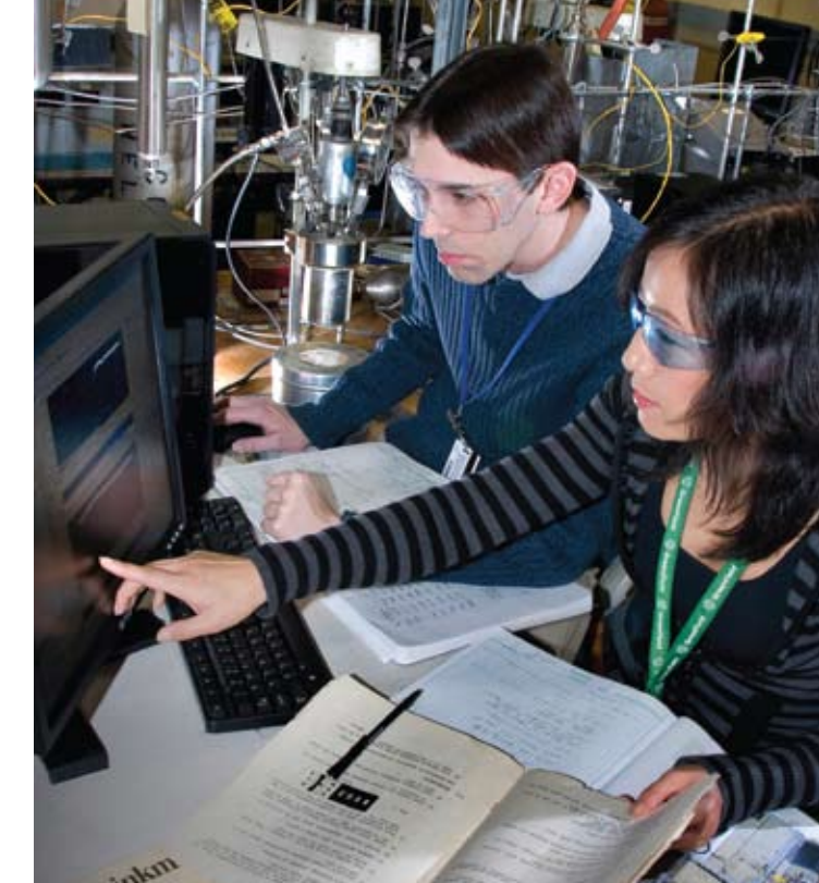
David Lacina and Weimin Zhou prepare a LabVIEW program to measure the hydrogen uptake and release from a complex hydride in solution.
