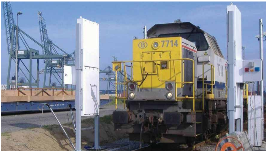
Radiation portal monitors along a rail line scan a train for the illicit trafficking of radioactive and special nuclear material.
