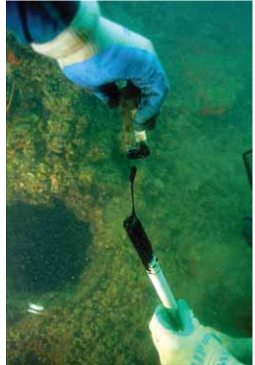
A sample of fuel oil is captured for laboratory research. NPS photo by Brett Seymour
