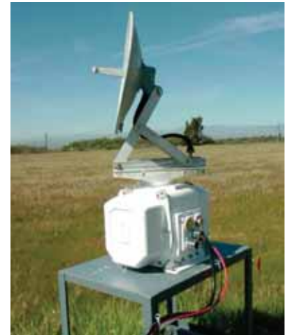
The BIRDRAD Furuno 2155BB radar transmitter-receiver with 24-inch parabolic antenna. The TR unit is mounted on a mobile cart and cables connect it to the black box unit in the utility trailer
