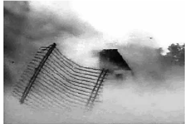
Historic-type iron perimeter gate becomes dangerous blast debris if not securely cabled to properly anchored fence. State Department blast test video furnished by the Protective Design Center.
