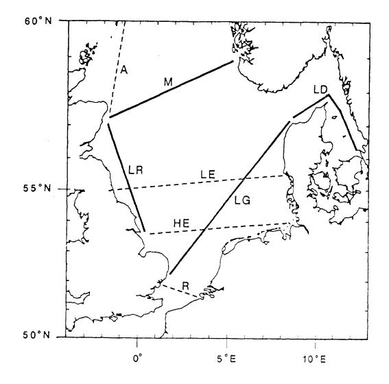
PLANKTON SAMPLING WITH THE CONTINUOUS PLANKTON RECORDER IN THE NORTH SEA DURING 1990. THE SOLID LINES ARE THE ROUTES WHICH CARRY INSTRUMENTATION... TEMPERATURE, DEPTH, CHLOROPHYLL, CONDUCTIVITY, TURBIDITY AND IRRADIANCE SENSORS FOR UPWELLING AND DOWNWELLING LIGHT.
